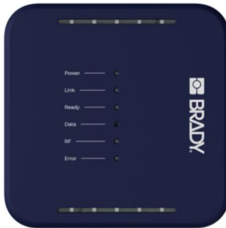
Figure 15: The placement of individual LEDs and the LED bars of the Brady IRX200
